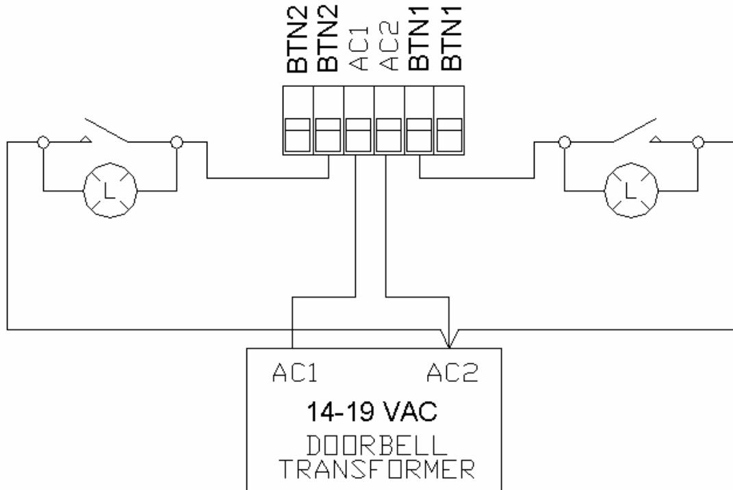
**Figure 3 - Single Button Wire – 2 Button Input**
