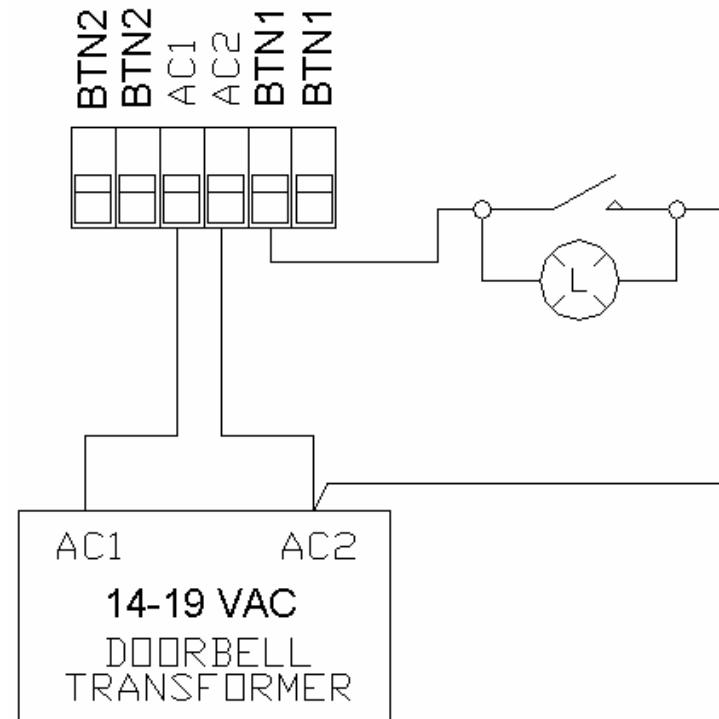
**Figure 4 – Single Button Wire – 1 Button Input**
