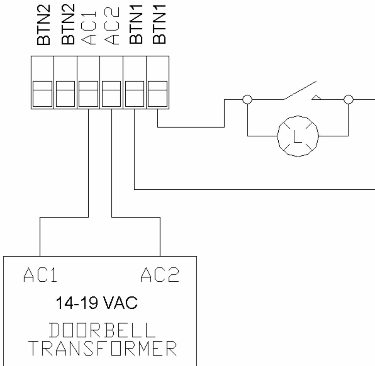
**Figure 2 – Preferred Wiring – 1 Button Input**
