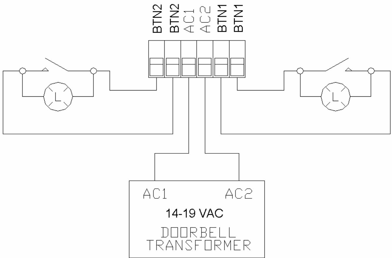
**Figure 1 – Preferred Wiring – 2 Button Input**
